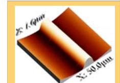
Figure 17: Teflon layer slowly decreasing in thickness towards waveguide. (Cheng & Kumar)
