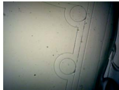
Figure 6: PDMS stamp with microdisk and waveguide negatives.
