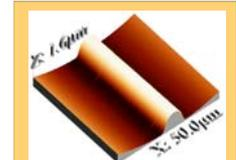
Figure 17: Teflon layer slowly decreasing in thickness towards waveguide. (Cheng & Kumar)
