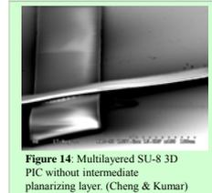
Figure 14: Multilayered SU-8 3D PIC without intermediate planarizing layer. (Cheng & Kumar)
