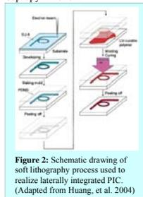
Figure 2: Schematic drawing of soft lithography process used to realize laterally integrated PIC. (Adapted from Huang, et al. 2004)
