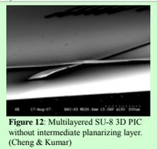
Figure 12: Multilayered SU-8 3D PIC without intermediate planarizing layer. (Cheng & Kumar)
