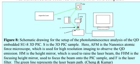
Figure 8: Schematic drawing for the setup of the photoluminescence analysis of the QD embedded SU-8 3D PIC. S is the 3D PIC sample. Here, AFM is the Nanonics atomic force microscope, which is used for high resolution imaging to observe the QD emission. HM is the height mirror, which is used to raise the laser beam, the FHM is the focusing height mirror, used to focus the beam onto the PIC sample, and F is the laser filter. The green line represents the laser beam path. (Cheng & Kumar)
