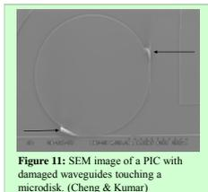
Figure 11: SEM image of a PIC with damaged waveguides touching a microdisk. (Cheng & Kumar)
