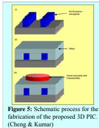
Figure 5: Schematic process for the fabrication of the proposed 3D PIC. (Cheng & Kumar)
