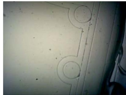
**Figure 6: PDMS stamp with microdisk and waveguide negatives.**
