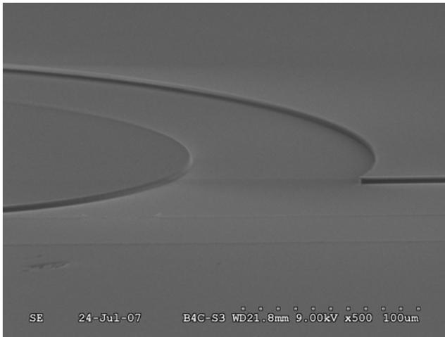
**Figure 7: SEM image of PIC with smooth sidewalls.**
